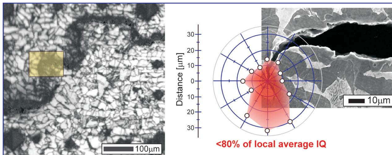
EBSD Image Quality (IQ) map of a secondary electron image of the highlighted area. Diagram of the low IQ area surrounding the crack tip, which is indicative of the local strain field. [4]
