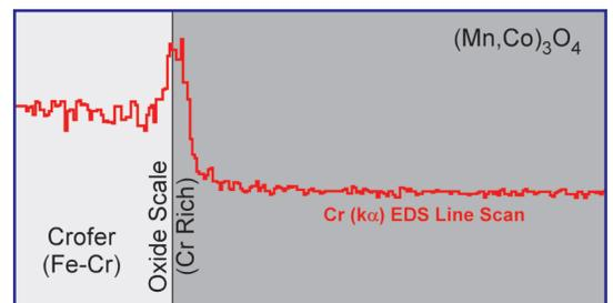
Schematic of a chromium EDS line scan of a post-tested SOFC showing minimal chromium migration from the stainless steel interconnect into the  $\text{Mn}_{1.5}\text{Co}_{1.5}\text{O}_4$  barrier coating. [8]
