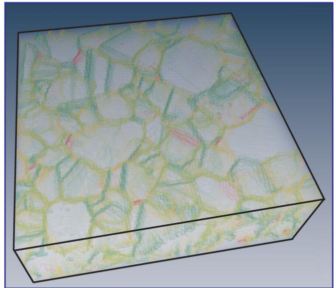
3D visualization of the grain boundary network in a nickel alloy measured by EBSD on a series of 2D sections. Grain boundaries are colored according to misorientation: from blue (low angle) to red (high angle).
